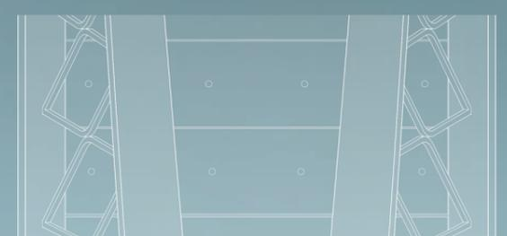
Beneath the deck the diagonals linking the deck and the lower chord are also in stainless steel. These bars, of varying sizes, are extremely compact, ranging from 65/65mm at the supports to 30/30mm in the middle of the bridge. As a result from a distance they will disappear which will emphasize the general outline of the structure.
