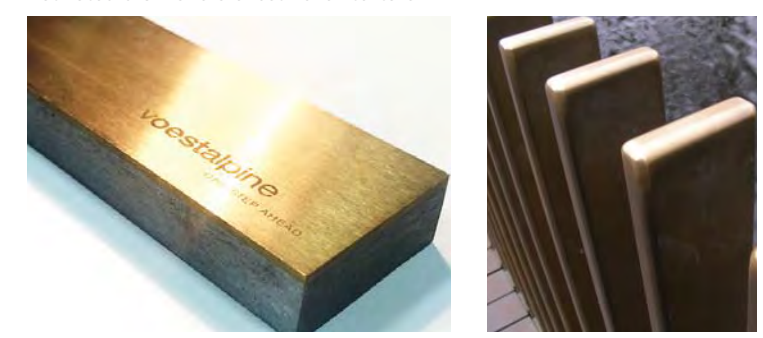
Steel plate roll bonded with 2mm phosphor bronze skin
